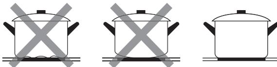
Make sure that the base of your pan is smooth, sits flat against the glass, and is the same size as the cooking zone. Use pans whose diameter is as large as the graphic of the zone selected. Using a pot a slightly wider energy will be used at its maximum efficiency. If you use smaller pot efficiency could be less than expected. Pot less than 140 mm could be undetected by the hob. Always centre your pan on the cooking zone.
