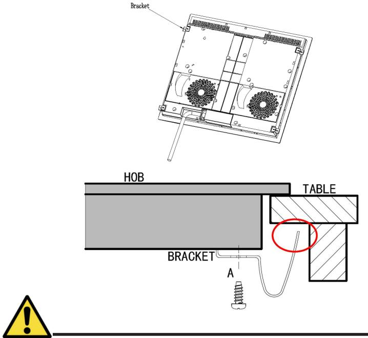
Under any circumstances, the brackets cannot touch with the inner surfaces of the worktop after installation (see picture).
