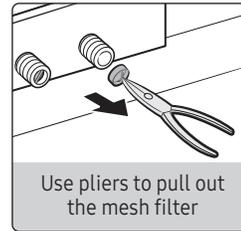
Use pliers to pull out the mesh filter
