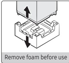
Use the machine without removing the foam bottom or the motor base (some models) causes the machine to malfunction and damage the internal components.
