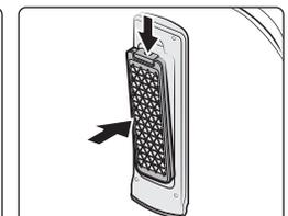
Reinsert the filter to the original position
